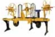
***Burying machine, deep injection up to 50cm, 3 injection shanks, bundled coils: Distance between shanks is adjustable: 0.60 to 1.4 m. NETAFIM™***
