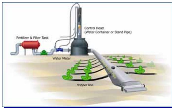
**Fig. 8.1 Low Pressure System components of Netafim™**
